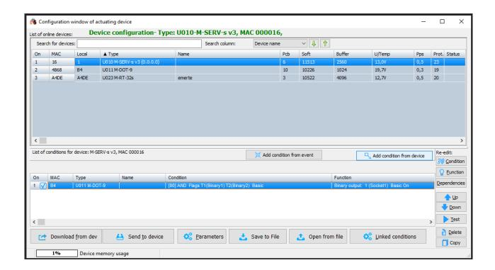
Tick the input to which a sensor is connected, e.g. motion sensor, set the Basic function and confirm.
