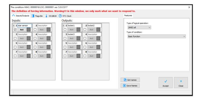
Tick the lamps that you want to control. Select the stair function and set the desired parameters:
