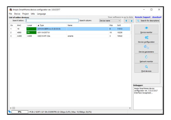
From the menu, choose an input device that will manage the operation (here, M-SERV-s again) and open Add condition from device.
