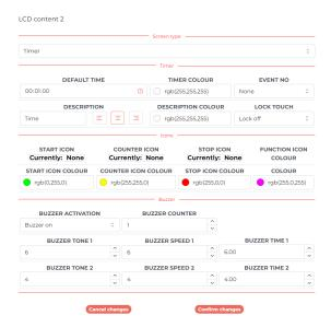
Next, in the M-DOT-M18 configuration menu, select the *Parameter -> LCD* tab, select the screen you want and select the "Access control" screen type, type in the "Description" field a message you want to display above the PIN input field.
