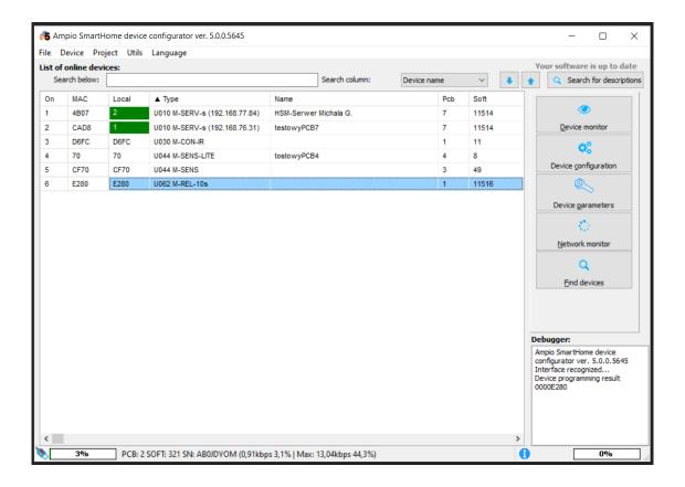
To begin with, go to *Device parameters*. For each of the relay outputs you can set up the function of a roller blinds output. Choose the right option from the dropdown list and save by clicking on *Send*.
